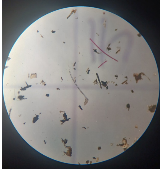
Figure 6: View of petri dish in stereoscope, with three microplastic fibers in view.
